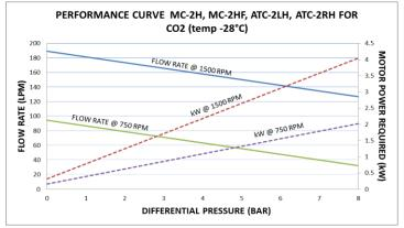
For liquids between 1-110 cP, predicted pump output will be the same as pump capacity chart on page 17. Actual pump output will be approximately 5-10% greater than predicted above.
