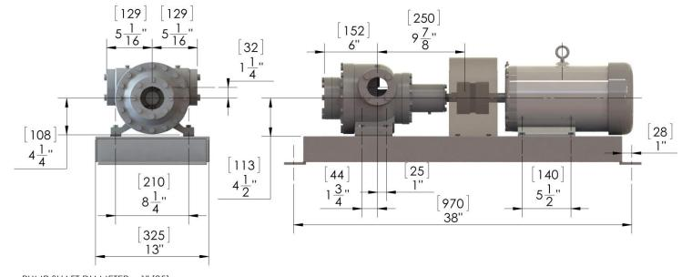
PUMP SHAFT DIAMETER = 1" [25] PUMP DRIVE SHAFT KEY SIZE 1/4" [6] X 1/4" [6] PUMP DRIVE SHAFT KEY SIZE 1/4" [6] X 1/4" [6] PUMP DIMENSIONS ARE FOR ATC-2L, ATC-2LH, ATC-2R, ATC-2RH PUMPS, 2-1/2" NPT INLET, 2" NPT OUTLET MOTOR SHAFT SIZE 1-1/8" [29] MOTOR DIMENSIONS ARE FOR 184T FRAME, 1800 RPM, 5 HP (3.7kW) MOTOR, OTHER FRAME SIZES AVAILABLE \* ALL DIMENSIONS  $\pm 1/16$  IN INCHES, [] DENOTES MM \*\*FOR A MORE DETAILED DRAWING, PLEASE VISIT SMITHPUMPS.COM
