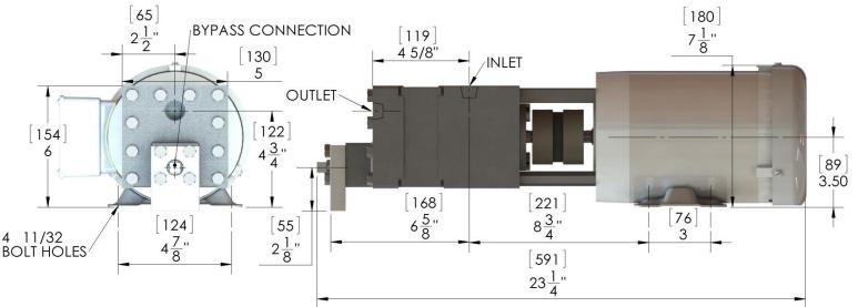
DIMENSIONS SHOWN ARE FOR 56-C FRAME MOTOR WITH FEET
