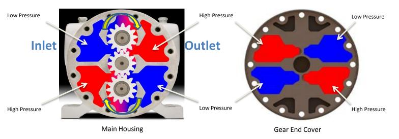
Liquid first enters the inlet of the pump, shown as blue in the upper left corner of the pump main housing. It is also directed within the pump to the bottom right port, also shown as blue through the porting in the gear end housing.
