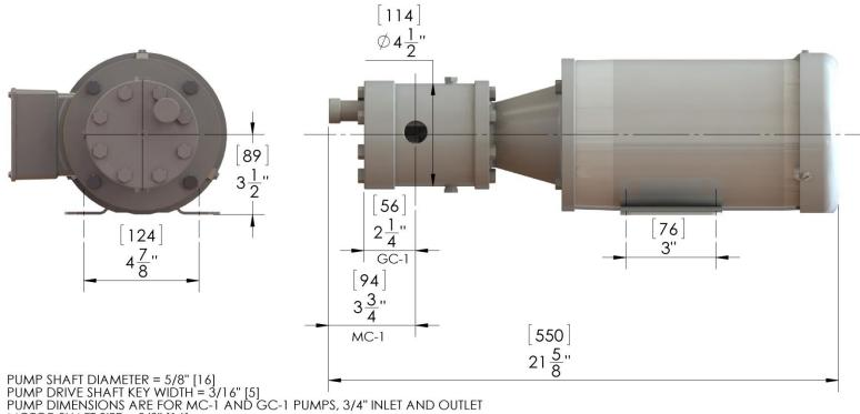
MOTOR SHAFT SIZE = 5/8" [16] MOTOR DIMENSIONS ARE FOR 56C FRAME MOTOR WITH FEET, 1 HP (.75 kW)
