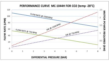
For liquids between 1-110 cP, predicted pump output will be the same as pump capacity chart on page 13. Actual pump output will be approximately 5-10% greater than predicted above.
