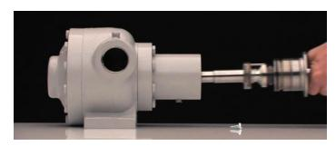
Old mechanical seal can be removed in the field in a matter of minutes! No disassembly of the pump required!
