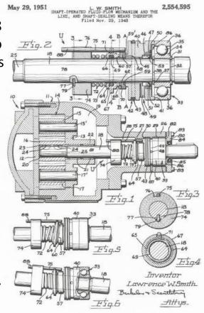
First patent issued for a mechanical seal used in a liquefied gas pump. Within seven years, most pumps were using mechanical seals.
