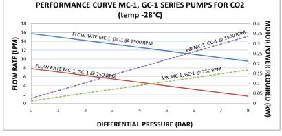
For liquids between 1-110 cP, predicted pump output will be the same as pump capacity chart on page 11. Actual pump output will be approximately 5-10% greater than predicted above.
