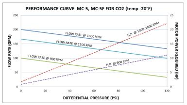
For liquids between 1-110 cP, predicted pump output will be the same as pump capacity chart on page 26. Actual pump output will be approximately 5-10% greater than predicted above. For 250 GPM, specify our "Large" gear option.
