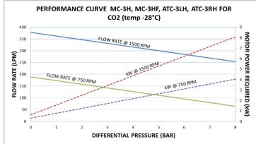
For liquids between 1-110 cP, predicted pump output will be the same as pump capacity chart on page 20. Actual pump output will be approximately 5-10% greater than predicted above.
