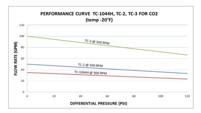
For liquids between 1-110 cP, predicted pump output will be the same as pump capacity chart on page 28. Actual pump output will be approximately 5-10% greater than predicted above.
