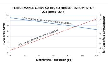
For liquids between 1-110 cP, predicted pump output will be the same as pump capacity chart on page 9. Actual pump output will be approximately 5-10% greater than predicted above.
