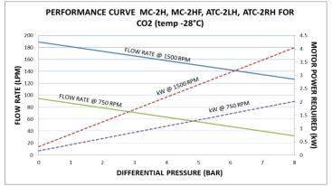
For liquids between 1-110 cP, predicted pump output will be the same as pump capacity chart on page 15. Actual pump output will be approximately 5-10% greater than predicted above.
