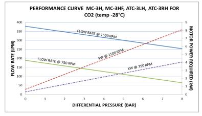
For liquids between 1-110 cP, predicted pump output will be the same as pump capacity chart on page 22. Actual pump output will be approximately 5-10% greater than predicted above.
