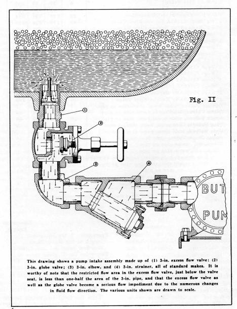
Now let us see how high the tank should be mounted if we use 2" pipe, valves, fittings, etc., instead of the 3" size. In such a case, we have, from Table 2:
