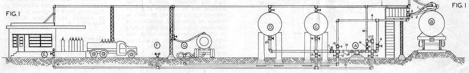
load truck and trailer transports, with double hoses as shown at station G. Correct valving for these and other operations will be apparent by referring to the drawing above.
