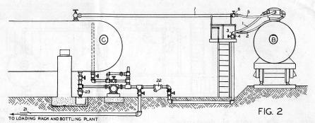
vapor is withdrawn through vapor line 7 from the storage tank C and discharged into R.R. tank B. The compressor alone is run until a differential pressure of approximately 10 lbs. is reached, after which the pump A at the storage tank is started. Even through this long line, the flow was very rapid and it was found that the speed of transfer more than doubled that which was obtainable with either pump or compressor operating separately.
