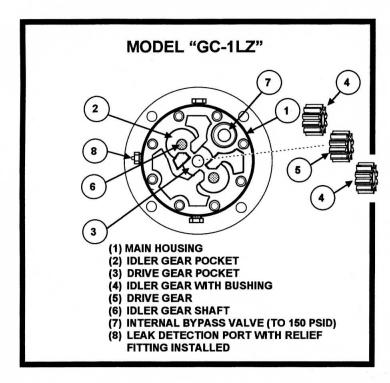
These drawings of this fractional HP motor-mounted Smith pump, model "GC-1LZ" (13 USGPM), show how supplied liquid is simultaneously directed into four pumping chambers. Each chamber is strategically positioned to maintain axial and radial forces at equilibrium, and also to reduce internal flow resistance. The flow path, illustrated to the right, proceeds as follows:
