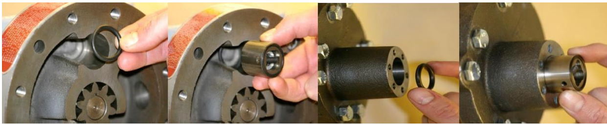
6227-17 o-ring inserted first into E-series main housing
