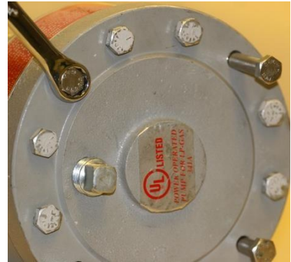
Remove 4 cap screws to separate the pump from the motor
