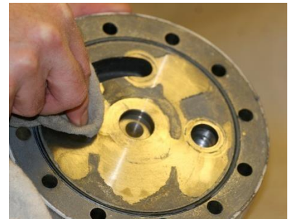
Old sealant being removed; a razor blade or any lubricant such as WD-40 can be used
