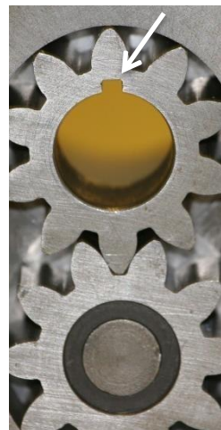
Replacement shaft seal assembly inserted into main housing with key in 12 o'clock position to fit drive gear keyway also in 12 o'clock position
