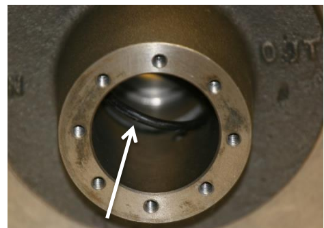
Remove the 6227-17 O-ring. The replacement shaft seal assembly comes with a new, replacement o-ring.
