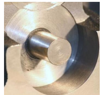
Idler gear shaft in good condition
