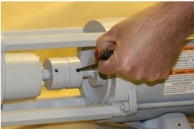
Tightening of coupling set screw using allen wrench
