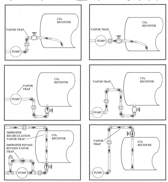
In addition to the most common sources of pump vapor lock problems illustrated, there are other potential sources of excessive suction line vaporization, which are less obvious.
