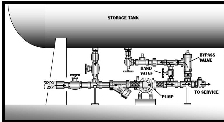
When the demand for product within the system exceeds the pump capacity, or if improper pressure equalization procedures are at play, this occurrence would attempt to turn the pump, independently, of its motor. This kind of energy utilization, and interference with the motor, causes an internal pressure drop.
