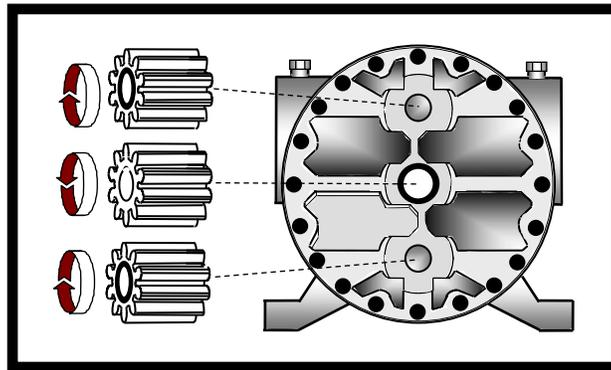
Smith pump gearing, as opposed to power transmission gearing, when applied to the transfer of liquids with low viscosity as liquefied gases, requires special attention to assume uniformity of surface finish, concentricity, parallelism, backlash, lubrication clearances, and bearing tolerances. Continually balanced internal loading afforded within the Smith pump can only be assured through application of superior wearing materials and even load distribution over relatively large areas .
