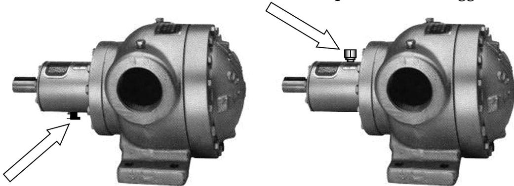
highly abrasive ice, or frozen product, building up around the seals, accelerating their failure. During this time, material will also be removed from the gear teeth, and the drive gear(s) will be dragged into the bottom of their respective bores, enlarging critical clearances beyond limitations, allowing for cavitation or vapor-lock and highly decreased pumping efficiency.
