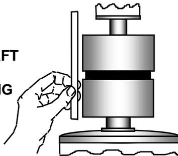
Fast coupling wear indicates misalignment of pump and motor shafts. Misalignment or the continued use of a worn coupling insert, can be responsible for rapid pump wear, continual seal leaks, and noise. The proper way to align the Smith drive coupling is shown in the sketch. (See Bulletin "AL-3").
