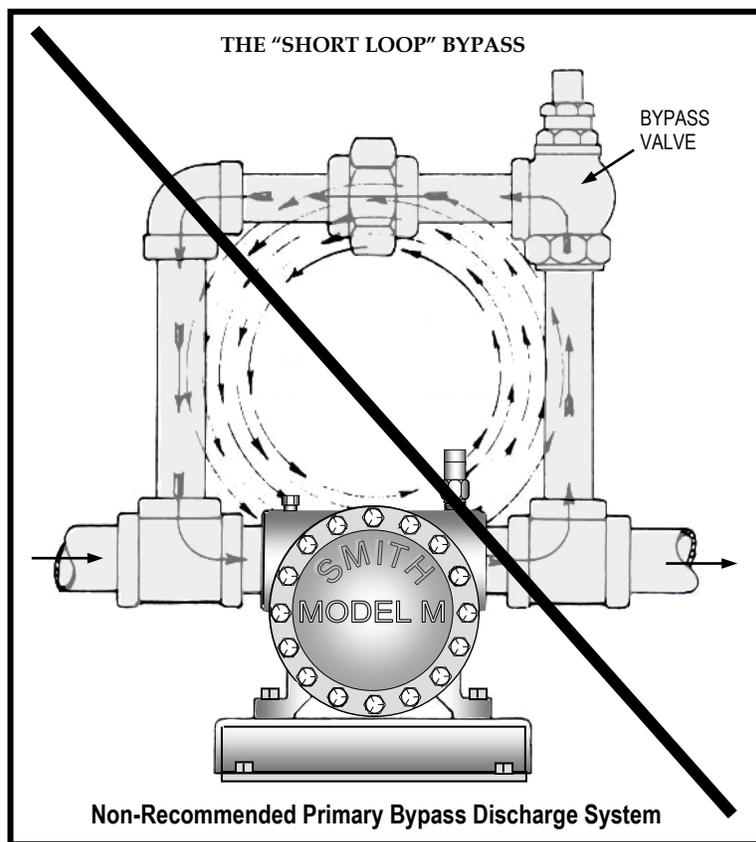
In many cases, returning the bypass to the supply tank actually benefits the operation by increasing the pressure of the liquid fed to the pump. The higher this pressure is, the less liquid displacement by vapor there will be, and the lower the differential pressure will have to be to transfer at the rate desired.
