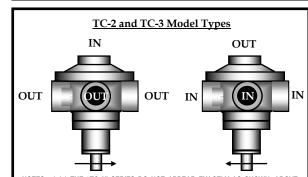
NOTES: (1) THE "TC-3" SERIES DO NOT APPEAR EXACTLY AS SHOWN, ABOVE. THEY HAVE A SECONDARY GEAR HOUSING INSTALLED BETWEEN THE GEAR END COVER AND MAIN HOUSING, AND ARE CORRESPONDINGLY GREATER IN LENGTH.
