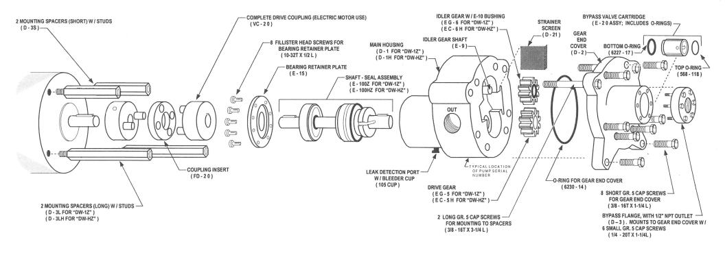
NOTES: (A) THESE PUMPS ARE PROVIDED WITH AN INTERNAL BYPASS VALVE WHICH MUST BE CONNECTED TO AN EXTERNAL LINE THROUGH THE 1/2" NPT PORT IN THE BYPASS FLANGE, MOUNTED TO THE GEAR END COVER. SEE OTHER AVAILABLE LITERATURE, OR CONTACT FACTORY FOR ADDITIONAL INFORMATION.
