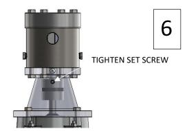
STEP 6: Now, tighten the pump coupling half set screw. As this is the last step in the procedure, do not forget to tighten the pump coupling half set screw.
