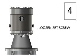
STEP 4: Now, loosen the set screw on the pump coupling half and push the pump down onto the face of the electric motor. This step will slightly push the pump coupling half into the correct position.
