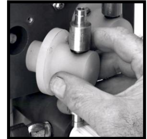
TYPICAL CHECK VALVE INSERT SIMILAR TO THOSE SHOWN TO THE LEFT, FOR PLASTIC MODEL R-1 (SOLD ONLY AS A 1:100/1:100 TWIN INJECTOR).
