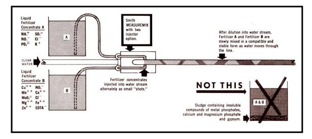
(3) SIMULTANEOUS INJECTION OF ACID AND NUTRIENT CHEMICALS WITHOUT COMBINING THEM PRIOR TO INJECTION. In most cases it is in the end user's best interests to always use a two-injector option when injecting acids. ALWAYS INJECT ACID BY ITSELF. DO NOT MIX IT WITH OTHER CHEMICALS. <u>THIS IS IMPORTANT</u>!
