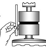
Fast coupling wear indicates misalignment of pump and motor shafts. Misalignment or the continued use of a worn coupling insert, can be responsible for rapid pump wear, continual seal leaks, and noise. The proper way to align the Smith drive coupling is shown in the sketch. (See Bulletin "AL-3").
