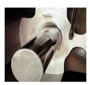
Checking for wear on the pocket ends.
