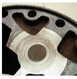
Normal gear end cover face with no functional wear.
