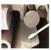
Checking for wear on the pocket diameters.
