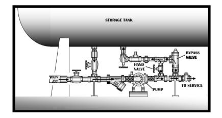
When the demand for product within the system exceeds the pump capacity, or if improper pressure equalization procedures are at play, this occurrence would attempt to turn the pump, independently, of its motor. This kind of energy utilization, and interference with the motor, causes an internal pressure drop.
